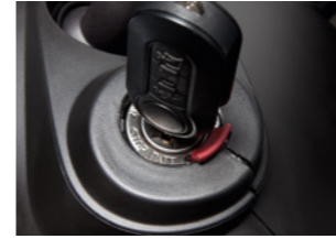
Cab battery isolation switch to prevent discharge in storage
